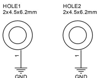
In TOP side a pad has diameter 180mil (accordance to top of screw).
