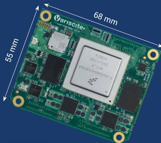
The SoM includes a variety of interfaces and connectivity options: Certified dual-band Wi-Fi 802.11 ac/a/b/g/n, BT/BLE, dual GbE, dual USB3, PCIe, SATA III, CAN, SPI and UART.
