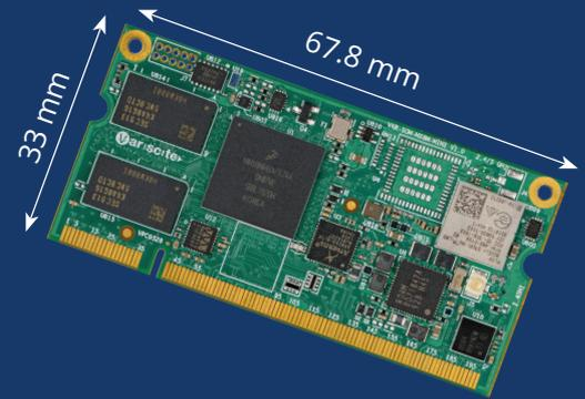
This popular platform supports a variety of interfaces including certified single band 802.11b/g/n as well as dual-band 802.11ac/a/b/g/n option, 5.2 BT/BLE, Gigabit Ethernet, CAN bus, dual USB2.0 and LVDS. Additionally, the SoM provides an integrated HW engines supporting 1080p video encoding/decoding, 2D and 3D GPU, HQ audio all in a full industrial range of -40 to 85°C and a generous longevity commitment of 15-years.
