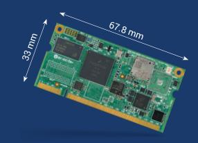
This popular platform supports a variety of interfaces including certified single-band 802.11b/g/n as well as dual-band 802.11ac/a/b/g/n option, 4.2 BT/BLE, Gigabit Ethernet, CAN/CAN-FD, USB2.0 and LVDS.
