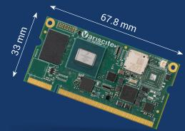
The VAR-SOM-MX8M-PLUS is a member of the VAR-SOM Pin2Pin product family, providing extensive scalability options and reduced development time, costs, and risks. Starting from i.MX 6UL/6ULL modules, through i.MX 6, i.MX 8M Nano, TI AM625x, i.MX 93, i.MX 8M Mini, up to i.MX 8X and i.MX 8QuadMax-based modules.
