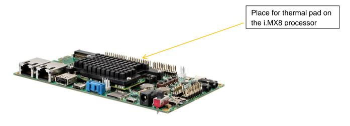
2.2 Assemble the heat spreader on top side of the VAR-SOM-MX8/X. Use the mechanical holes in order to align the heat spreader to VAR-SOM-MX8/X PCB.
