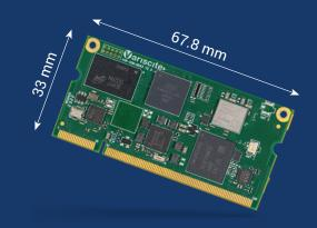
options and reduced development time, costs, and risks. Starting from i.MX 6UltraLite platforms, through the i.MX 6, i.MX 8M processors family and Tl's AM625x, up to the high-performance i.MX 8X and i.MX 8QuadMax platforms.
